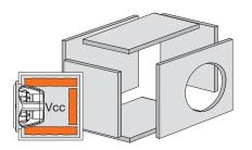
**Damping material:** FONOFORM on all the inside walls except for the speaker's.
